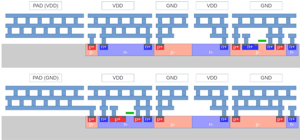
Simplified cross-sectional layout of PADVDD and PADGND cells
